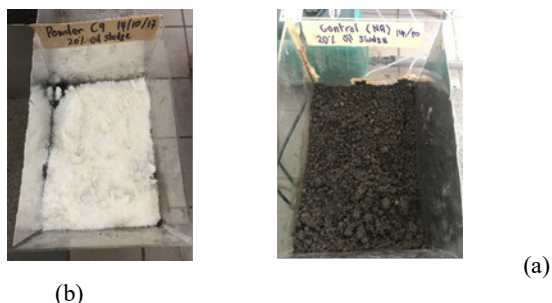
Fig 2. Biodegradation of oil sludge contaminated soil by (a) LIBeM-POW and (b) NA within 56 days.
